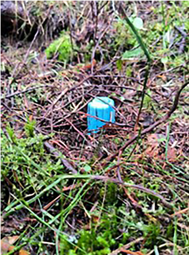
Fig. S1. Drill & Drop Bluetooth probe (Sentek Technologies) installed on one of the study plots to record soil moisture and temperature up to 30 cm depth
